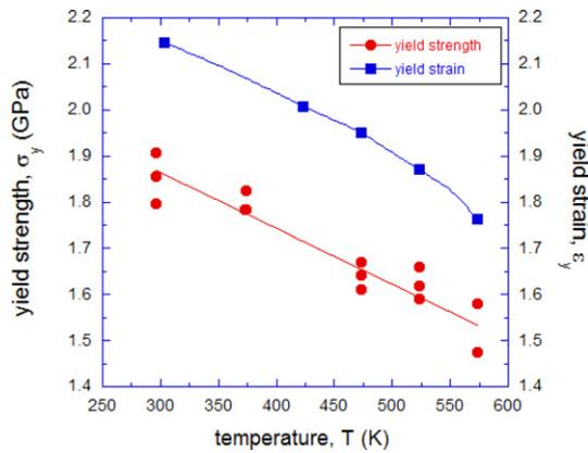
**Figure 2.** Variation of yield strength,  $\sigma_y$ , and yield strain,  $\epsilon_y$ , as a function of temperature. The  $\sigma_y$  data are taken from Lu et al. [7] and the strain rate effects are neglected.
