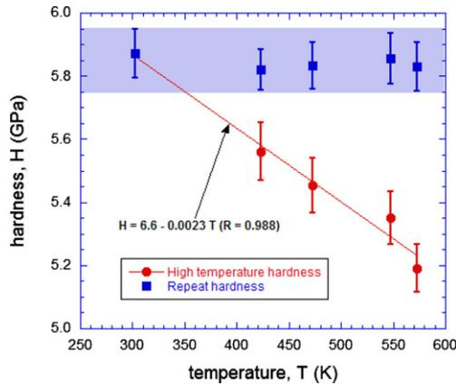
**Figure 1.** Plot showing the variation of Vickers hardness,  $H$ , with temperature. Also plotted are the room hardness values, measured after the high temperature exposure, as a function of the temperature of exposure.
