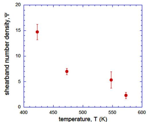
Figure 6. Variation of shear band number density (calculated on per indent basis) as a function of temperature.
