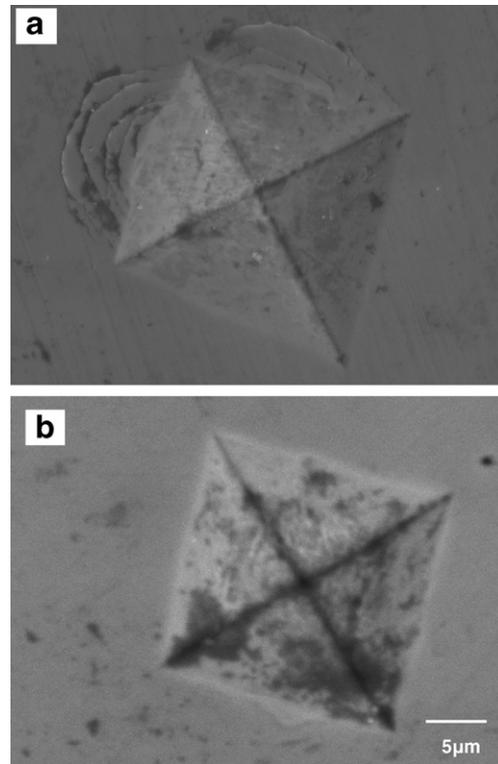
Figure 5. Typical Vickers indentation impressions obtained at (a) 423 K and (b) 573 K.
