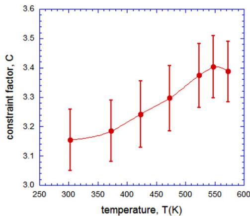
**Figure 3.** Variation of the constraint factor,  $C$ , given by the  $H/\sigma_y$  ratio, as a function of temperature.
