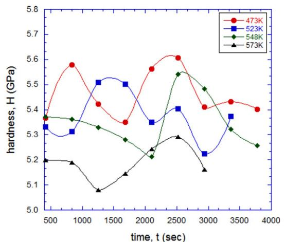
**Figure 4.** Sequential variation of hardness values as a function of time at temperature during high temperature indentation tests.
